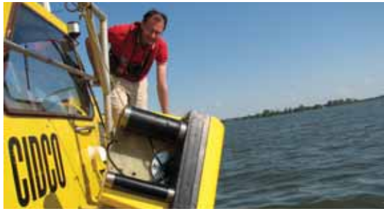
Figure 2: Left: Reson 7125 SV 30° starboard tilted. Right: CIDCO's survey vessel.
