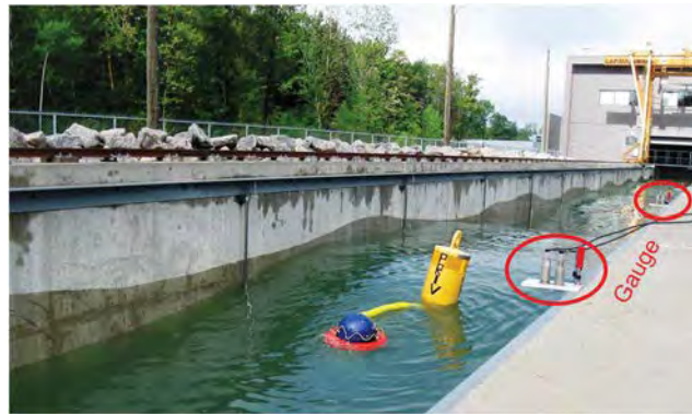
Figure 4. Wave measurement in INRS's hydraulic flume using the HydroBall ® . [Colour online.]
